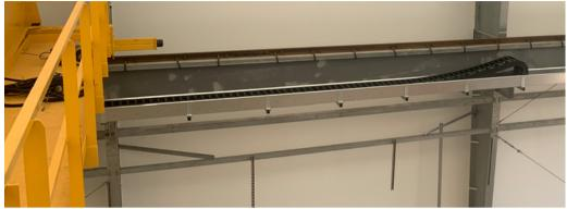
WHILE TYPICALLY USED FOR THE TROLLEY MOTION, CABLE CHAINS CAN BE EMPLOYED FOR THE BRIDGE MOTION WHEN THE CRANE CONTROLS ARE NOT MOUNTED ON THE CRANE.
